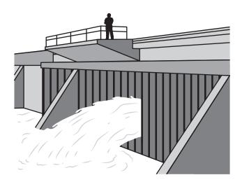
When the river level gets dangerously high, the spillway is opened. Opening the spillway lowers the water level in the Mississippi River.
